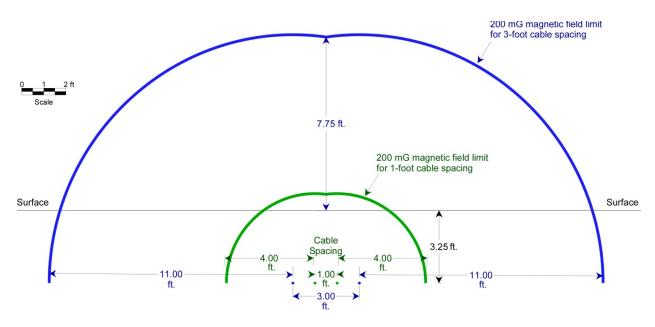
Figure 5.1.14-1. 200-mG Magnetic Field Strengths with Cable Spacings of 1 Foot and 3 Feet
